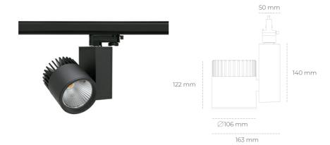
COB 2000 [K] MEAT PINK Light colour CRI Led chip flux 1845 [lm] Luminous flux 1476 [lm] System power 21 [W] Luminaire Efficiency 70 [lm/W] Beam angle 60° Controller ON/OFF MacAdam 3 SDCM
