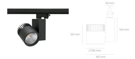
COB 2000 [K] MEAT PINK Light colour CRI Led chip flux 1741 [lm] Luminous flux 1392 [lm] System power 19 [W] Luminaire Efficiency 73 [Im/W] Beam angle 15° Controller ON/OFF MacAdam 3 SDCM
