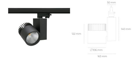
COB Light colour 3000 [K] | CRI Led chip flux 2767 [lm] Luminous flux 2213 [lm] System power 23 [W] Luminaire Efficiency 96 [lm/W] Beam angle 20° Controller ON/OFF MacAdam 3 SDCM
