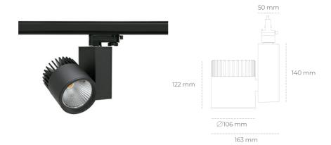
COB Light colour 2700 [K] | CRI 4000 [lm] Led chip flux Luminous flux 3200 [lm] System power 35 [W] Luminaire Efficiency 91 [lm/W] Beam angle 15° Controller ON/OFF MacAdam 3 SDCM
