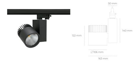
COB Light colour 2700 [K] | CRI Led chip flux 1111 [lm] Luminous flux 888 [lm] System power 10 [W] Luminaire Efficiency 89 [lm/W] Beam angle 15° Controller ON/OFF MacAdam 3 SDCM
