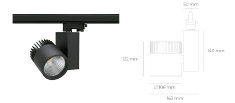
COB Light colour 5000 [K] | CRI Led chip flux 1447 [lm] Luminous flux 1157 [lm] System power 10 [W] Luminaire Efficiency 116 [lm/W] Beam angle 20° Controller ON/OFF MacAdam 3 SDCM
