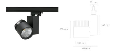
COB Light colour 4000 [K] | CRI Led chip flux 4542 [lm] Luminous flux 3633 [lm] System power 31 [W] Luminaire Efficiency 117 [lm/W] Beam angle 45° Controller ON/OFF MacAdam 3 SDCM
