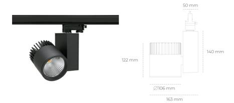
COB Light colour 4000 [K] | CRI Led chip flux 3122 [lm] Luminous flux 2497 [lm] System power 21 [W] Luminaire Efficiency 119 [lm/W] Beam angle 20° Controller ON/OFF MacAdam 3 SDCM
