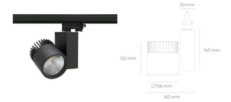
COB Light colour 3500 [K] | CRI Led chip flux 2783 [lm] Luminous flux 2226 [lm] System power 19 [W] Luminaire Efficiency 117 [lm/W] Beam angle 60° Controller ON/OFF MacAdam 3 SDCM
