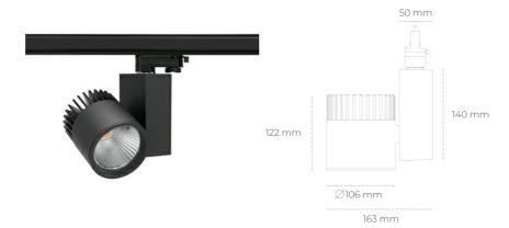
COB Light colour 3500 [K] | CRI Led chip flux 1948 [lm] Luminous flux 1558 [lm] System power 14 [W] Luminaire Efficiency 111 [lm/W] Beam angle 60° Controller ON/OFF MacAdam 3 SDCM
