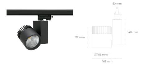
COB Light colour 3500 [K] | CRI 5010 [lm] Led chip flux Luminous flux 4008 [lm] System power 35 [W] Luminaire Efficiency 115 [lm/W] Beam angle 30° Controller ON/OFF MacAdam 3 SDCM
