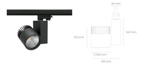
COB Light colour 3500 [K] | CRI Led chip flux 4453 [lm] Luminous flux 3562 [lm] System power 31 [W] Luminaire Efficiency 115 [lm/W] Beam angle 30° Controller ON/OFF MacAdam 3 SDCM
