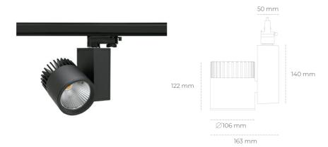
COB Light colour 3000 [K] | CRI Led chip flux 3538 [lm] Luminous flux 2830 [lm] System power 25 [W] Luminaire Efficiency 113 [lm/W] Beam angle 45° Controller ON/OFF MacAdam 3 SDCM
