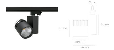
COB Light colour 3000 [K] | CRI Led chip flux 4355 [lm] Luminous flux 3484 [lm] System power 31 [W] Luminaire Efficiency 112 [lm/W] Beam angle 20° Controller ON/OFF MacAdam 3 SDCM
