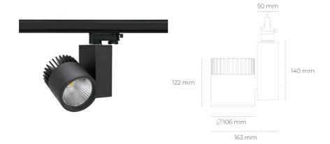
COB Light colour 2700 [K] | CRI Led chip flux 3502 [lm] Luminous flux 2801 [lm] System power 25 [W] Luminaire Efficiency 112 [lm/W] Beam angle 20° Controller ON/OFF MacAdam 3 SDCM
