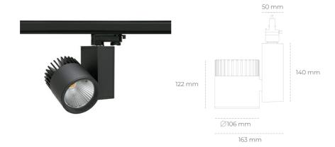
COB 3000 [K] PREMIUM COLOR Light colour CRI 90 Led chip flux 2776 [lm] Luminous flux 2220 [lm] System power 25 [W] Luminaire Efficiency 89 [lm/W] Beam angle 60° Controller ON/OFF MacAdam 3 SDCM
