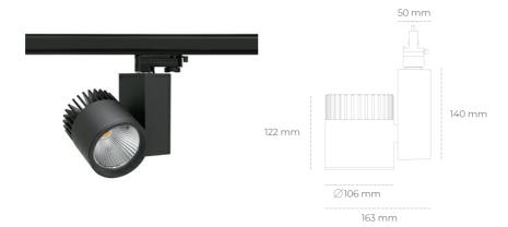
COB 3000 [K] PREMIUM COLOR Light colour CRI 90 Led chip flux 3827 [lm] Luminous flux 3061 [lm] System power 37 [W] Luminaire Efficiency 83 [lm/W] Beam angle 30° Controller ON/OFF MacAdam 3 SDCM
