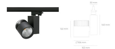
COB 3000 [K] CRI97 Light colour CRI Led chip flux 2402 [lm] Luminous flux 1921 [lm] System power 21 [W] Luminaire Efficiency 91 [lm/W] Beam angle 60° Controller ON/OFF MacAdam 3 SDCM
