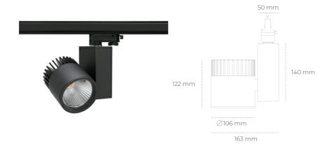
COB 3000 [K] CRI97 Light colour CRI 3368 [lm] Led chip flux Luminous flux 2694 [lm] System power 31 [W] Luminaire Efficiency 87 [lm/W] Beam angle 15° Controller ON/OFF MacAdam 3 SDCM
