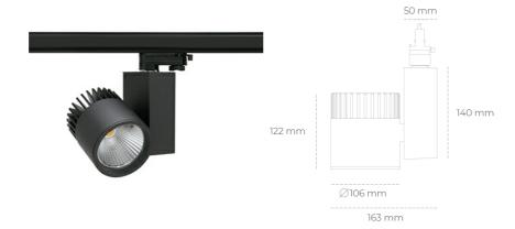
COB 3500 [K] PREMIUM WHITE Light colour CRI 90 Led chip flux 3245 [lm] Luminous flux 2596 [lm] System power 21 [W] Luminaire Efficiency 124 [lm/W] Beam angle 45° Controller ON/OFF MacAdam 3 SDCM
