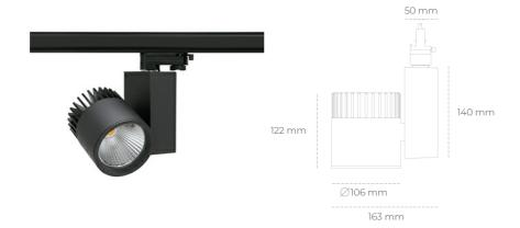
COB 3000 [K] PREMIUM WHITE Light colour CRI 90 Led chip flux 3659 [lm] Luminous flux 2927 [lm] System power 25 [W] Luminaire Efficiency 117 [lm/W] Beam angle 30° Controller ON/OFF MacAdam 3 SDCM
