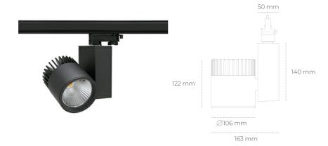
COB 3000 [K] PREMIUM WHITE Light colour CRI 90 Led chip flux 1497 [lm] Luminous flux 1197 [lm] System power 11 [W] Luminaire Efficiency 109 [lm/W] Beam angle 30° Controller ON/OFF MacAdam 3 SDCM
