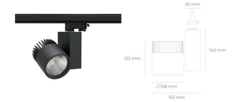
COB 4200 [K] MEAT WHITE Light colour CRI 90 Led chip flux 2519 [lm] Luminous flux 2015 [lm] System power 25 [W] Luminaire Efficiency 81 [lm/W] Beam angle 60° Controller ON/OFF MacAdam 3 SDCM
