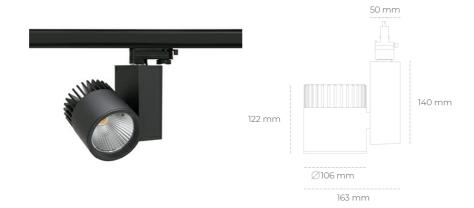
COB 4200 [K] MEAT WHITE Light colour CRI 90 Led chip flux 2159 [lm] Luminous flux 1727 [lm] System power 21 [W] Luminaire Efficiency 82 [lm/W] Beam angle 60° Controller ON/OFF MacAdam 3 SDCM
