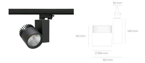
COB 4200 [K] MEAT WHITE Light colour CRI 90 Led chip flux 3375 [lm] Luminous flux 2700 [lm] System power 35 [W] Luminaire Efficiency 77 [Im/W] Beam angle 45° Controller ON/OFF MacAdam 3 SDCM
