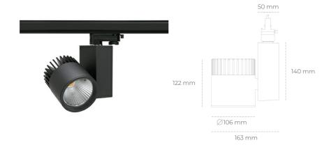
COB 4200 [K] MEAT WHITE Light colour CRI 90 Led chip flux 2340 [lm] Luminous flux 1872 [lm] System power 23 [W] Luminaire Efficiency 81 [lm/W] Beam angle 15° Controller ON/OFF MacAdam 3 SDCM
