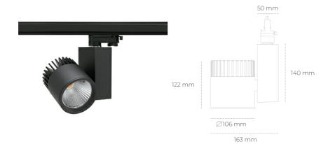
COB 4000 [K] HI EFFICIENT Light colour CRI 90 Led chip flux 5532 [lm] Luminous flux 4425 [lm] System power 34 [W] Luminaire Efficiency 130 [lm/W] Beam angle 60° Controller ON/OFF MacAdam 3 SDCM
