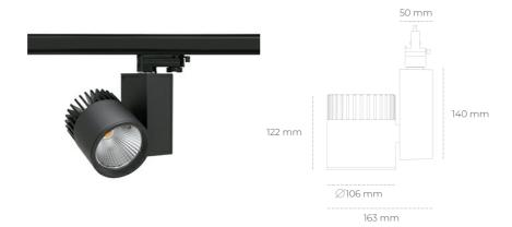
COB 4000 [K] HI EFFICIENT Light colour CRI 90 Led chip flux 4090 [lm] Luminous flux 3272 [lm] System power 25 [W] Luminaire Efficiency 131 [lm/W] Beam angle 20° Controller ON/OFF MacAdam 3 SDCM
