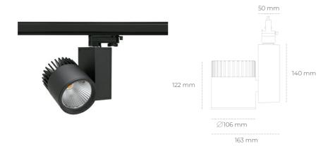
COB 4000 [K] HI EFFICIENT Light colour CRI 90 Led chip flux 1625 [lm] Luminous flux 1300 [lm] System power 10 [W] Luminaire Efficiency 130 [lm/W] Beam angle 20° Controller ON/OFF MacAdam 3 SDCM
