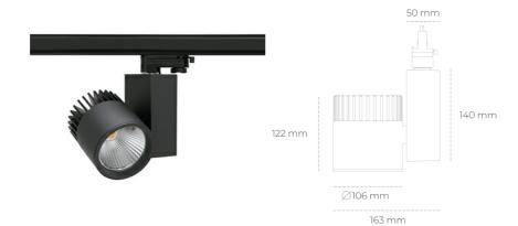
COB 3500 [K] HI EFFICIENT Light colour CRI 90 Led chip flux 3341 [lm] Luminous flux 2672 [lm] System power 21 [W] Luminaire Efficiency 127 [lm/W] Beam angle 15° Controller ON/OFF MacAdam 3 SDCM
