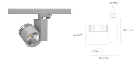
COB 2500 [K] BREAD Light colour CRI 4299 [lm] Led chip flux Luminous flux 3439 [lm] System power 37 [W] Luminaire Efficiency 93 [lm/W] Beam angle 20° Controller ON/OFF MacAdam 3 SDCM
