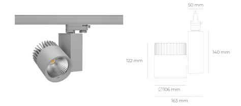
COB 2500 [K] BREAD Light colour CRI 3042 [lm] Led chip flux Luminous flux 2433 [lm] System power 25 [W] Luminaire Efficiency 97 [lm/W] Beam angle 20° Controller ON/OFF MacAdam 3 SDCM
