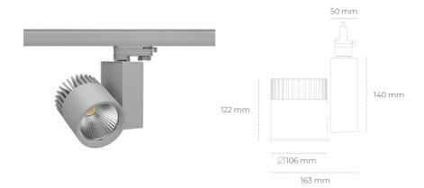
COB 2500 [K] BREAD Light colour CRI Led chip flux 2574 [lm] Luminous flux 2059 [lm] System power 21 [W] Luminaire Efficiency 98 [lm/W] Beam angle 20° Controller ON/OFF MacAdam 3 SDCM
