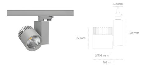
COB 2000 [K] MEAT PINK Light colour CRI Led chip flux 2807 [lm] Luminous flux 2245 [lm] System power 35 [W] Luminaire Efficiency 64 [lm/W] Beam angle 60° Controller ON/OFF MacAdam 3 SDCM
