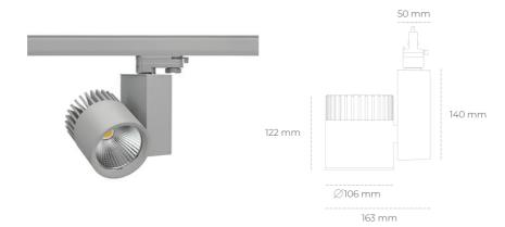
COB 2000 [K] MEAT PINK Light colour CRI Led chip flux 1845 [lm] Luminous flux 1476 [lm] System power 21 [W] Luminaire Efficiency 70 [lm/W] Beam angle 45° Controller ON/OFF MacAdam 3 SDCM
