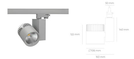
COB Light colour 4000 [K] | CRI 2899 [lm] Led chip flux Luminous flux 2319 [lm] System power 23 [W] Luminaire Efficiency 101 [lm/W] Beam angle 20° Controller ON/OFF MacAdam 3 SDCM
