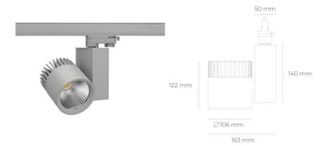
COB Light colour 2700 [K] | CRI Led chip flux 2667 [lm] Luminous flux 2133 [lm] System power 23 [W] Luminaire Efficiency 93 [lm/W] Beam angle 60° Controller ON/OFF MacAdam 3 SDCM
