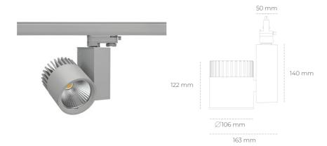
COB Light colour 4000 [K] | CRI Led chip flux 4542 [lm] Luminous flux 3633 [lm] System power 31 [W] Luminaire Efficiency 117 [lm/W] Beam angle 60° Controller ON/OFF MacAdam 3 SDCM
