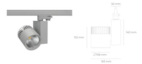
COB Light colour 4000 [K] | CRI Led chip flux 3122 [lm] Luminous flux 2497 [lm] System power 21 [W] Luminaire Efficiency 119 [lm/W] Beam angle 45° Controller ON/OFF MacAdam 3 SDCM
