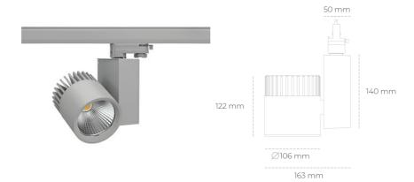
COB Light colour 3500 [K] | CRI 3896 [lm] Led chip flux Luminous flux 3116 [lm] System power 27 [W] Luminaire Efficiency 115 [lm/W] Beam angle 20° Controller ON/OFF MacAdam 3 SDCM
