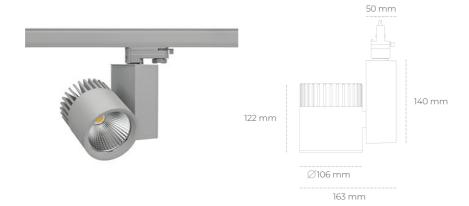
COB Light colour 3000 [K] | CRI Led chip flux 4355 [lm] Luminous flux 3484 [lm] System power 31 [W] Luminaire Efficiency 112 [lm/W] Beam angle 60° Controller ON/OFF MacAdam 3 SDCM
