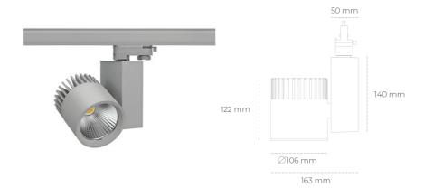
COB Light colour 3000 [K] | CRI Led chip flux 2994 [lm] Luminous flux 2395 [lm] System power 21 [W] Luminaire Efficiency 114 [lm/W] Beam angle 45° Controller ON/OFF MacAdam 3 SDCM
