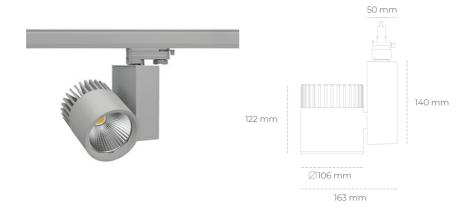
COB Light colour 3000 [K] | CRI Led chip flux 3538 [lm] Luminous flux 2830 [lm] System power 25 [W] Luminaire Efficiency 113 [lm/W] Beam angle 20° Controller ON/OFF MacAdam 3 SDCM
