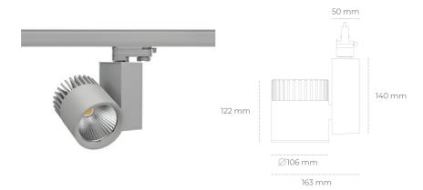
COB Light colour 3000 [K] | CRI Led chip flux 4355 [lm] Luminous flux 3484 [lm] System power 31 [W] Luminaire Efficiency 112 [lm/W] Beam angle 15° Controller ON/OFF MacAdam 3 SDCM
