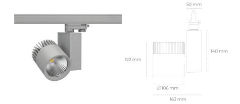
COB Light colour 3000 [K] | CRI Led chip flux 2994 [lm] Luminous flux 2395 [lm] System power 21 [W] Luminaire Efficiency 114 [lm/W] Beam angle 15° Controller ON/OFF MacAdam 3 SDCM
