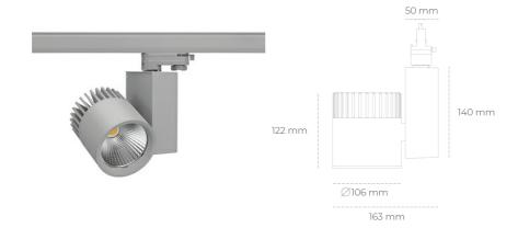
COB Light colour 2700 [K] | CRI Led chip flux 3772 [lm] Luminous flux 3017 [lm] System power 27 [W] Luminaire Efficiency 112 [lm/W] Beam angle 45° Controller ON/OFF MacAdam 3 SDCM
