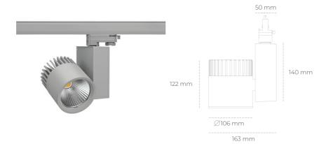
COB Light colour 2700 [K] | CRI Led chip flux 3502 [lm] Luminous flux 2801 [lm] System power 25 [W] Luminaire Efficiency 112 [lm/W] Beam angle 15° Controller ON/OFF MacAdam 3 SDCM
