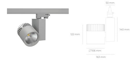
COB 4000 [K] PREMIUM WHITE Light colour CRI 90 Led chip flux 4764 [lm] Luminous flux 3811 [lm] System power 37 [W] Luminaire Efficiency 103 [lm/W] Beam angle 60° Controller ON/OFF MacAdam 3 SDCM
