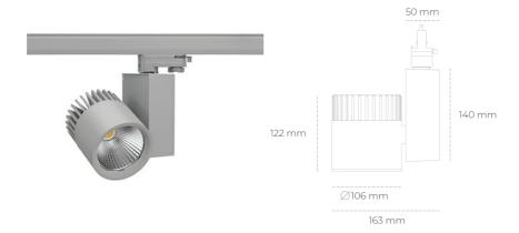
COB 4000 [K] PREMIUM WHITE Light colour CRI 90 Led chip flux 1887 [lm] Luminous flux 1509 [lm] System power 14 [W] Luminaire Efficiency 108 [lm/W] Beam angle 30° Controller ON/OFF MacAdam 3 SDCM
