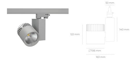
COB 3000 [K] PREMIUM COLOR Light colour CRI 90 Led chip flux 1145 [lm] Luminous flux 916 [lm] System power 11 [W] Luminaire Efficiency 83 [lm/W] Beam angle 60° Controller ON/OFF MacAdam 3 SDCM
